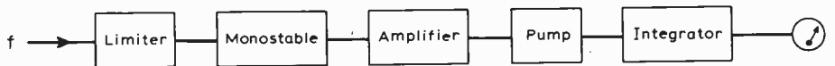
Fig. 2. Input signal is processed to feed constant-amplitude and constant-width pulses to the diode-transistor pump.
